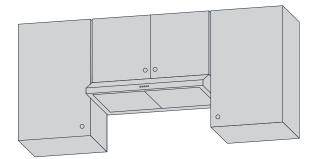
Carefully hang the hood on the mounting screws in place from Step 2. The bottom of the hood should match up with the horizontal line marked on the wall.
