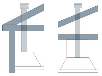
Or, vent through a side wall if you cannot vent directly above your hood. You can also install your insert over a kitchen island and vent it through the ceiling, as in the picture below.
