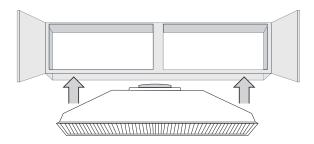
• Gently lift the range hood insert inside the custom hood or cabinetry. Ask a friend to help so you can attach the duct in step 3.
