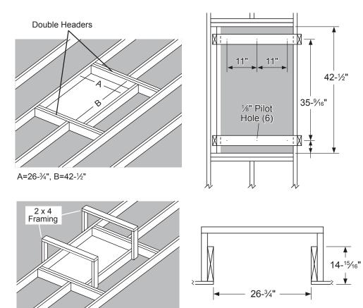
The hood must be centered over the cooktop. Make sure there is enough room in your ceiling for the 44" hood and its ductwork. For the best performance, mount your hood between 36" and 72" above the cooktop. You may need to cut the joists in your ceiling to make room for this frame.
