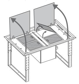
2. Remove the two interior panels by unscrewing eight screws from each panel.
