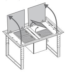
2. Remove the two interior panels by unscrewing eight screws from each panel.
