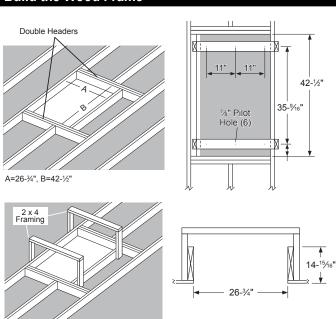
The hood must be centered over the cooktop. Make sure there is enough room in your ceiling for the 44" hood and its ductwork. For the best performance, mount your hood between 36" and 72" above the cooktop. You may need to cut the joists in your ceiling to make room for this frame.
